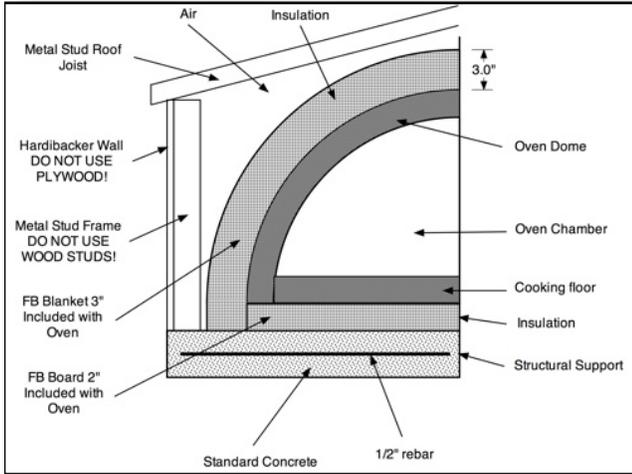
10.2. The layers of a walled enclosure oven.
