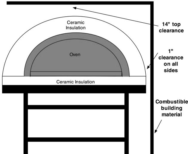
The oven must have a minimum 1" (25 mm) clearance to combustibles from all sides, and 14" (356 mm) clearance to combustibles from the top.
